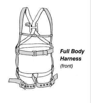
The fall-arrest system must be adequately anchored. That means anchored to something that will support the weight of a small car (about 3600 lbs.). Fall arrest loads can be high.
